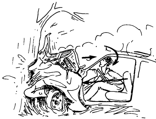
FIG. 9—Mechanism of hangman's fracture in motor-vehicle frontal impact. Extension, axial loading, and shear of upper cervical spine.
